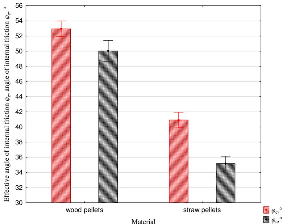
Fig. 5. Angle of internal friction and effective angle of internal friction depending on type of pellets
