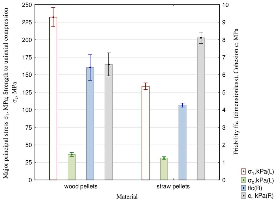
Fig. 4. Friction parameters depending on type of pellets
