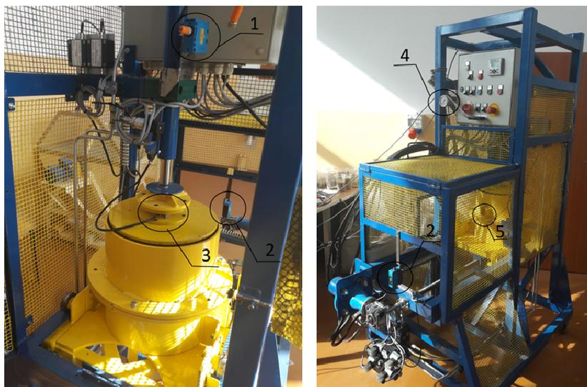
**Fig. 1. View of test bench to determine angle of internal friction. 1 – sensor of material displacement by compacting piston, 2 – sensor of cylinder displacement 3 – sensor of compacting force, 4 – sensor of oil pressure in the actuator, 5 – sensor of shear force**
