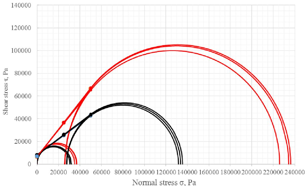
Fig. 3. Linear flow conditions for two types of pellets
